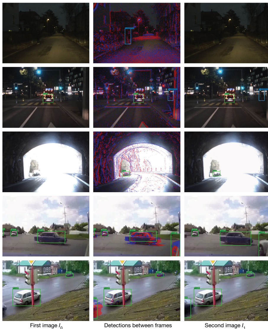
Fig. 5 | Qualitative results of the proposed detector for edge-case scenarios. The first column shows detections for the first image I_0 . The second column shows detections between images I_0 and I_1 using events. The third column
