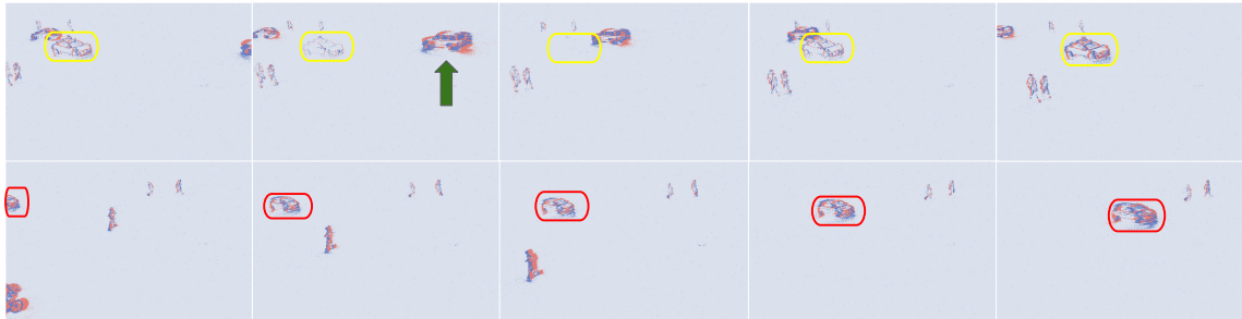
Figure 6.1: Demonstrating Effectiveness Of Event Camera For Traffic Scenarios: Yellow Circle (Top Row) Tracks A Car That Halts At A Stop Sign With Lack Of Motion Captured In The Third Frame, Red Circle (Bottom Row) Tracks A Car That Violates The Stop Sign Where Motion Is Continuously Captured In Every Frame. Additionally, The Green Arrow (Top Row) Shows A Car Traveling At A High Speed, Resulting In A High Event Density.
