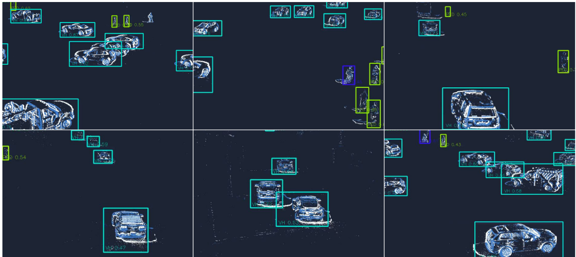
Figure 4.1: Traffic Participant Object Detection By RVT. Snapshots Illustrating The Detection Results Of RVT At Various Traffic Sites, Showcasing Its Performance In Diverse Real-world Scenarios.
